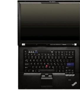
Lenovo ThinkPad T400. **Processor:** Intel® Core™ 2 Duo, **Processor code:** P8700, **Processor speed:** 2,53 GHz. **Screen size:** 35,8 cm (14.1"), **Screen resolution:** 1440 x 900 **Screen ratio:** 16:10. **Memory:** 2 GB, **Memory type:** DDR3-SDRAM. **Storage:** 320 GB. **Graphics:** AMD Mobility Radeon HD 3470. **Operating system:** Windows 7 Professional. **Weight:** 2,38 kg
